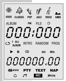
nnn:nnn In standby mode: displays the time. In tuner mode: displays the preset station. In MP3/WMA mode: displays the total number of albums and files, and the elapsed playing time of the current file. In CD-DA mode: displays the total playing time, and the elapsed
